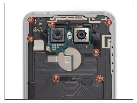
Remove the seven Phillips screws holding down the upper antenna shield.
