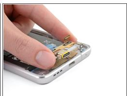
Use the flat end of an opening tool to pry up the USB-C / mic assembly and remove it from the phone.
