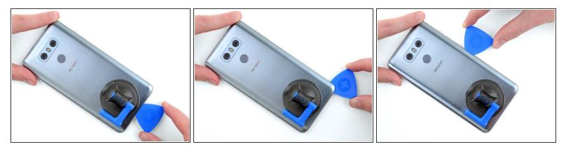
Re-insert the opening pick into the bottom edge of the phone and slide it up the right edge of the phone, cutting through the adhesive holding it in place.
