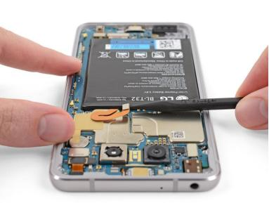
Use a spudger to pry up the press connector at the end of the battery's ribbon cable, disconnecting the battery.
