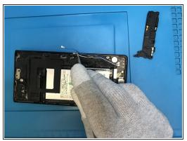
Use the point of a plastic spudger to lift the antenna cable connector up off of its socket on the logic board.
