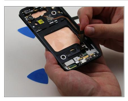
Pull the ribbon cable attached to the screen away from the board and make sure it is bent upwards and out of the way.
