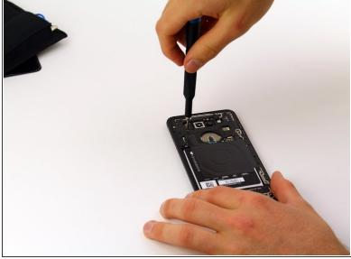
Remove the ten 4mm screws using the Phillips #00 Screwdriver.
