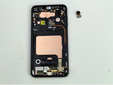
Use a Spudger to pry away the front-facing camera from the board.
