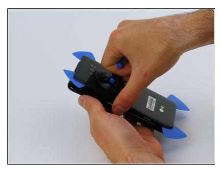
Once all edges of the device are lifted free, use a Suction Handle to gently pull the rear glass off the device.
