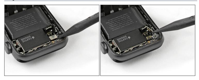
Use the point of a pry tool to disconnect the Force Touch gasket by prying its connector straight up.
