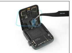
• Use a pair of tweezers to gently remove the blue protective liner on top of the Force Touch gasket, exposing the last of the adhesive.
