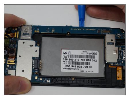
Gently pull up and remove the motherboard using the iFixit opening tool.
