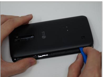
Using an iFixit opening tool, gently pull outward on the cutout on the bottom left corner of the phone to remove the back cover.
