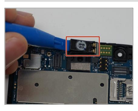
Gently pull the speaker out from its compartment with the iFixit opening tool.
