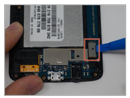
Disconnect the flex cable from the motherboard with the iFixit opening tool.
