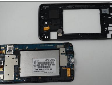
Gently remove the mid-frame using an iFixit opening tool as shown.
