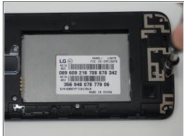
Remove the nine 2mm JIS #00 screws from the mid-frame.
