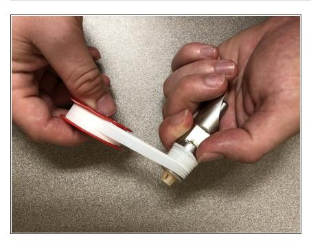
Use Teflon tape to line the threads of the new nipple.
