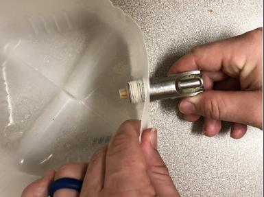
Place the new nipple in the hole with the peg on top.
