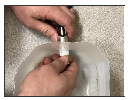
Place and thread the nut on the inside of the container on the backside of the nipple.
