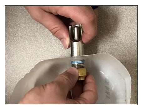
With an adjustable wrench, unscrew the nut on the inside located near the base on the backside of the nipple.
