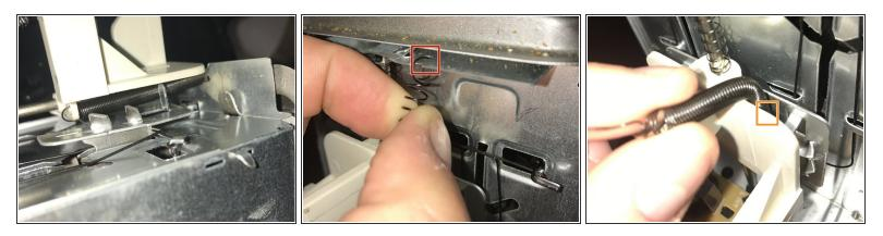
Re sure to remember where the spring is attached to prevent frustration putting the new spring on.
