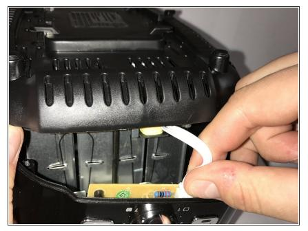
• Disconnect the wire shown in the picture. After disconnecting the wire, proceed to take the cover off.
