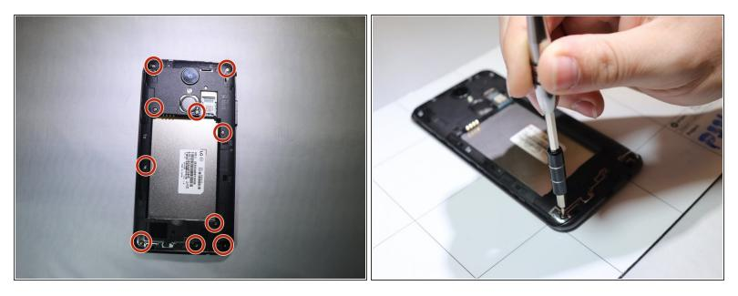
• Use your PH000 screwdriver to remove the ten 1.4mm x 4mm screws.
