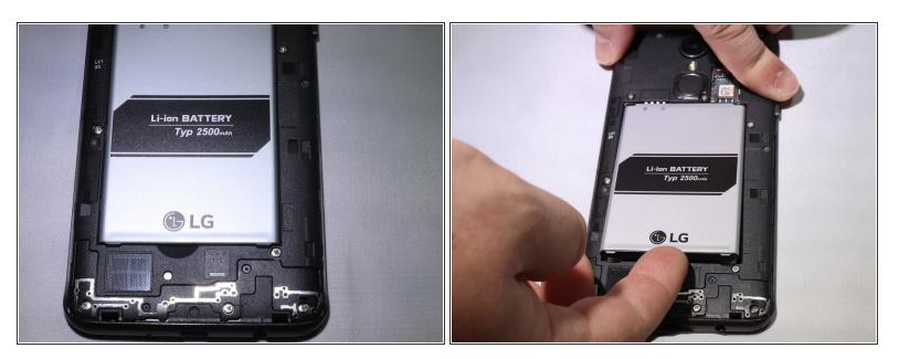
• Use the slot in the middle of the bottom edge of the battery to pry it up and out of the case.
