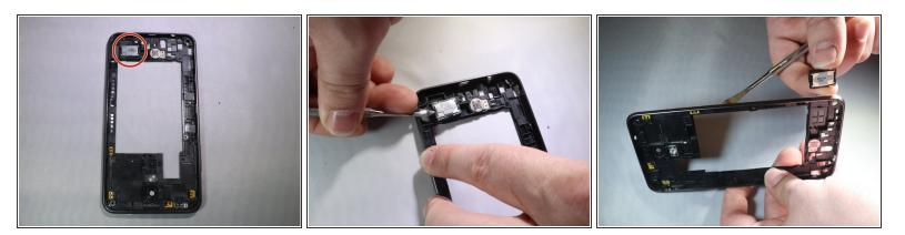
Using the metal spudger lift up and remove the speaker along with the magnetic tape it comes with.
