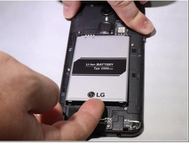
Use the slot in the middle of the bottom edge of the battery to pry it up and out of the case.
