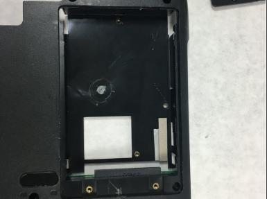
The hard drive is connected to the computer; simply pull it back from the connector and take it out
