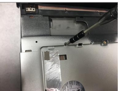
• Using the Phillips #0 screwdriver, remove the two 5mm screws that are highlighted to get access to the internal area of the laptop.
