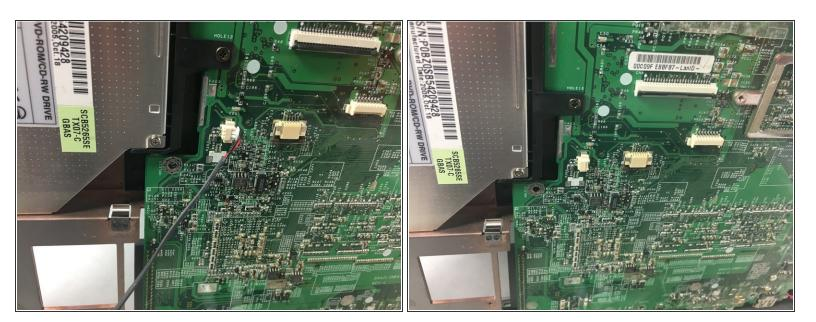
Flip the laptop over again and unplug the black and red cable from its socket. The display will come off entirely when the cables are removed.
