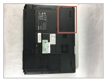
Locate the hard drive access panel in the upper right corner of the laptop.
