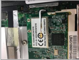
To completely remove the display, flip back over to the other side of the laptop. and unplug the two black and white coaxial cables.
