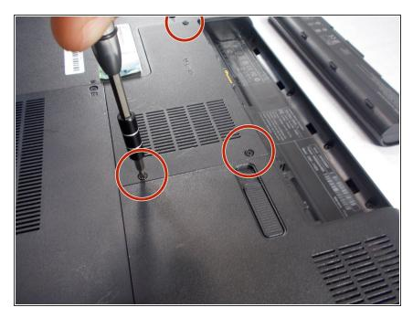
Unscrew the three 3mm screws on the compartment underneath the battery.
