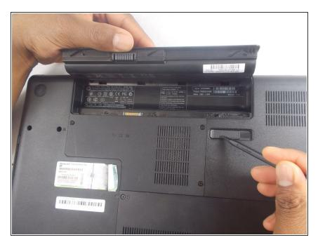
Remove the battery by pushing the switch to the left and removing the battery from its slot.
