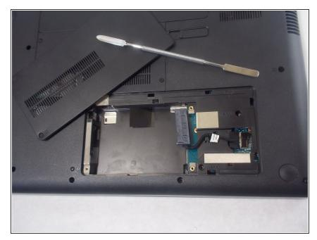
Use a Metal Spudger remove the panel. Underneath is where the hard drive is connected.
