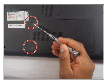
Use a Phillips screwdriver to remove the two 3mm screws on the lowest compartment.
