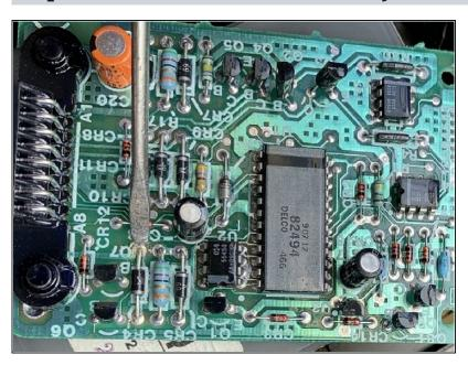
The tip of the screw driver is at the joint that has failed.
