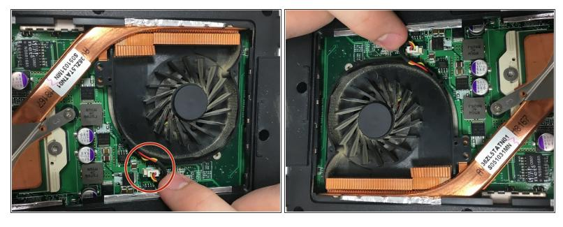
Disconnect the fan power cable from the motherboard by pulling the cable up and out of the connector.
