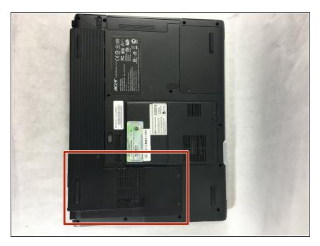
The panel you will be removing to access the internal fan is located at the bottom of the laptop.
