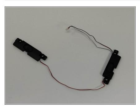
Lift the speakers from the case being careful of the wires connecting them. Put them to the side.
