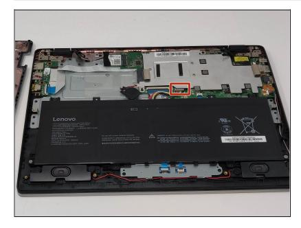
• For safety reasons, disconnect the wires connecting the battery to the motherboard with a nylon spudger.
