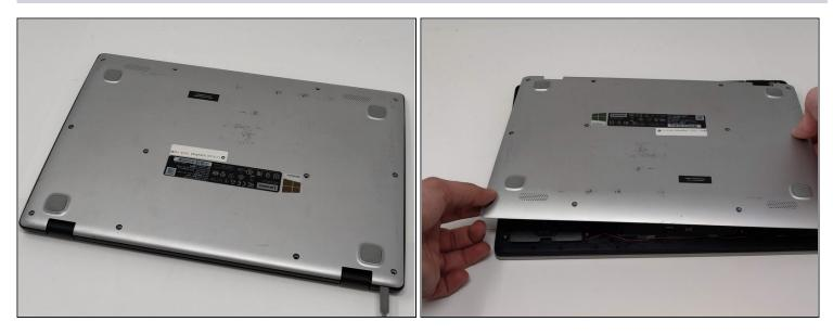
• Use the nylon spudger to loosen the back cover from the back of the device.
