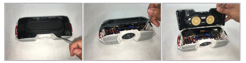
• Pry open the glued inner shell using a spudger around all sides of the shell.
