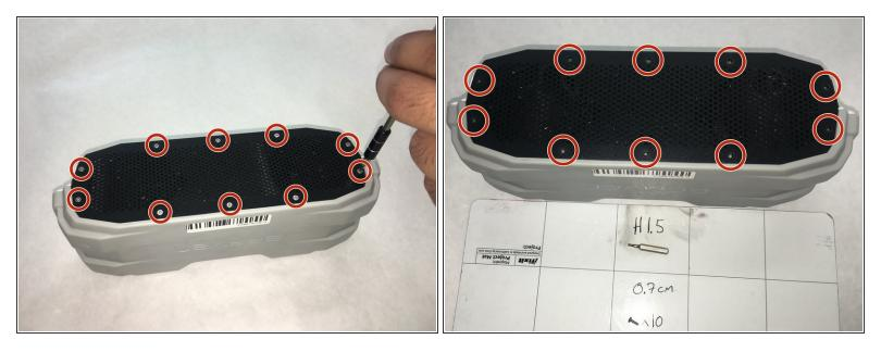
• Remove ten 0.7 cm screws in the front plate using the 1.5 mm Hex screwdriver.
