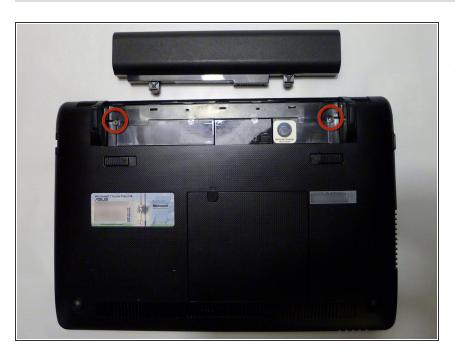
Remove screws on the battery compartment.
