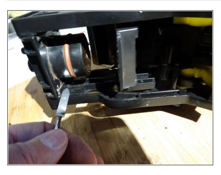
The upper piston is held in place in the frame with four locking pawls.
