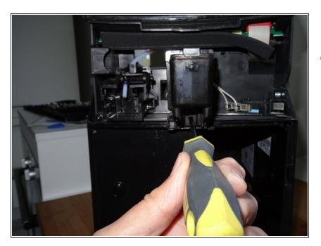
Remove the Torx T10 screws below the coffee distribution unit.
