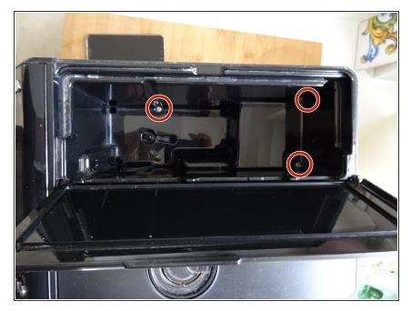
• Remove the three Torx T10 screws under the water tank.
