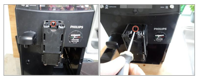
• Remove the Torx T10 screw at the top edge of the coffee dispensing spout.
