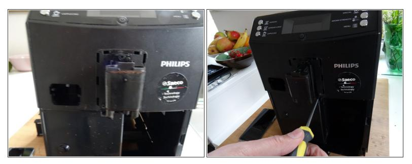
• Remove the Torx T10 screw at the lower edge of the coffee spout.
