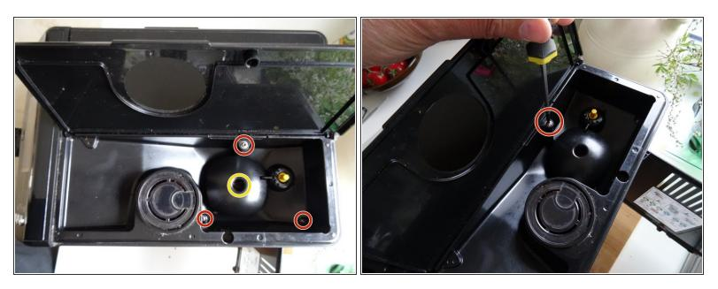
• Remove the Torx T20 screw on the finger guard of the grinder. Remove the finger guard.
