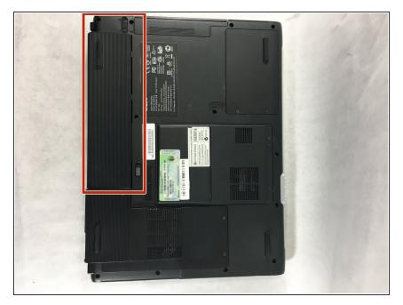
Turn the Acer Aspire 3003WLCi so that the bottom of the laptop is facing up. Orient it so that the battery is on your left.
