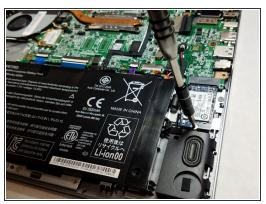
Remove the single 3mm screw holding the SSD with the Phillips #0 screwdriver.
