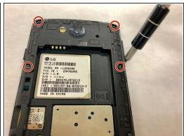
Use the Phillips #000 Screwdriver to remove the eight 4mm screws.
