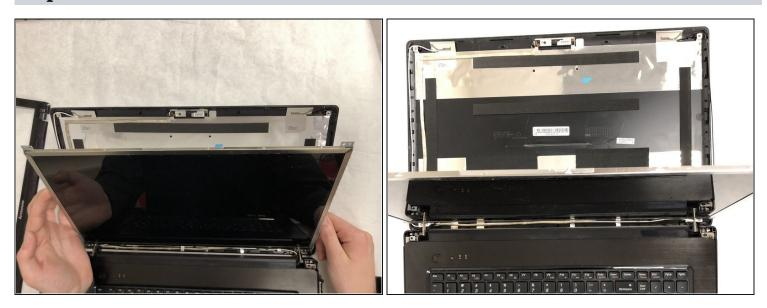
• With the back cover being removed from the screen frame, the back cover can be set aside.
