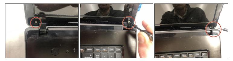
Using a Phillips #1 screwdriver, remove both 5.5mm screws from the corners of the screen.
