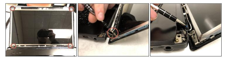
• Remove the four 8.5mm screws on the corners of the screen that connect the screen frame to the back cover.
