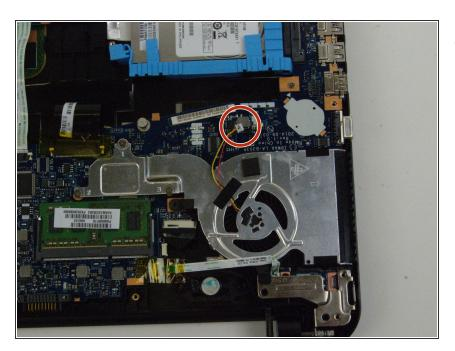
Disconnect the fan wire from the motherboard.
