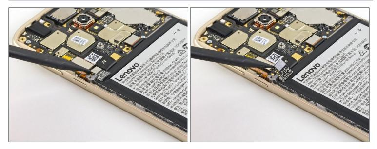
• Use the point of a spudger to pry up and disconnect the battery connector.
