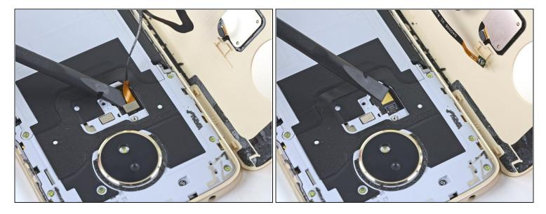
• Use a spudger to pry up and disconnect the fingerprint sensor cable connector.
