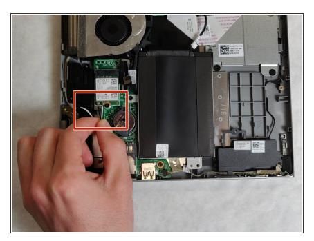
Unhook both of the wires attached to the WLAN adaptor.
