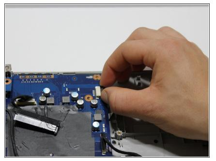
• Pull out the plastic cover to release the Kotl strip, then pull out the strip.
