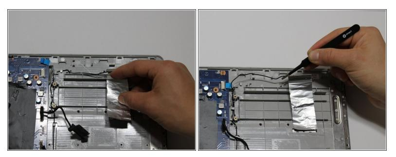
Gently pull up the aluminum strip from the top right corner of the computer and unthread the wire from the holders using the tweezers, without crimping the wire or tearing the aluminum.
