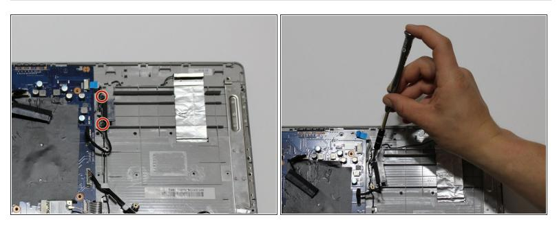
Using the J0 Japanese Industrial Standard screwdriver, remove the two 7mm screws that hold down the plug-in to the disc drive.
