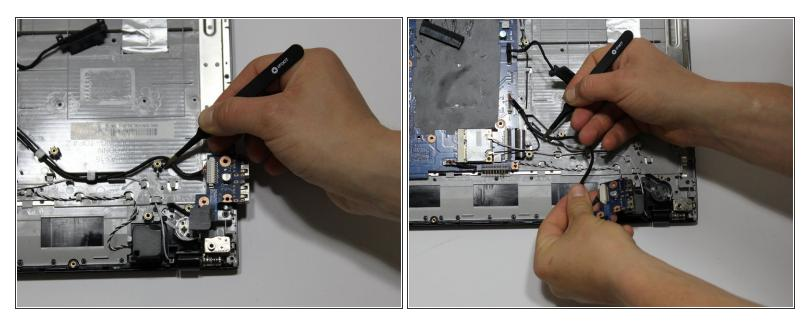
Using the tweezers, gently pry up the chip and ports, and unthread the wire from its holders, without crimping the wires.
