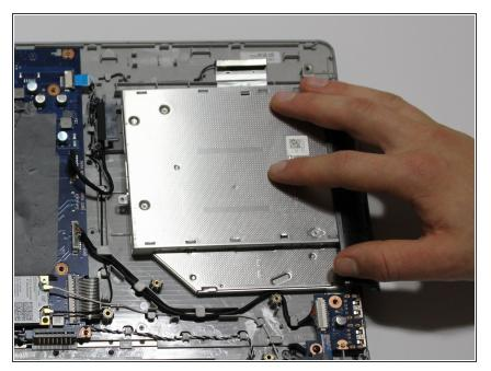
• Remove the disc drive by pulling it towards the outside of the computer.
