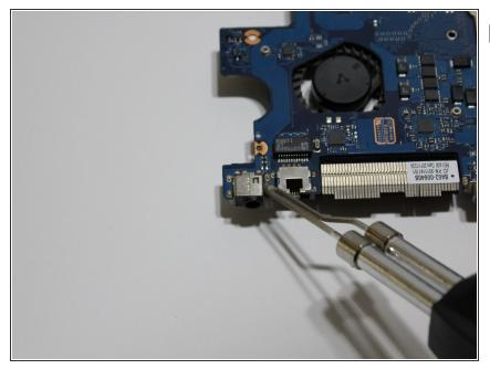
Solder the new power jack in place by reattaching the four connectors.
