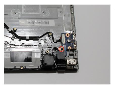
Using the J0 Japanese Industrial Standard screwdriver, remove the 3.5mm screw from the chip connected to the USB ports.
