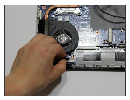
Disconnect the wire screen connection from its port by pulling upwards.
