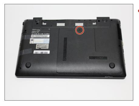
Using the J0 Japanese Industrial Standard screwdriver, remove the 4.5mm screw on the ODD/HDD Memory panel.
