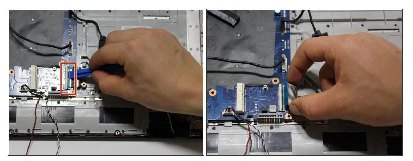
Using the iFixit opening tool, gently pry up the plastic clasp that holds the keyboard power circuit down, and pull out the strip from the connection.
