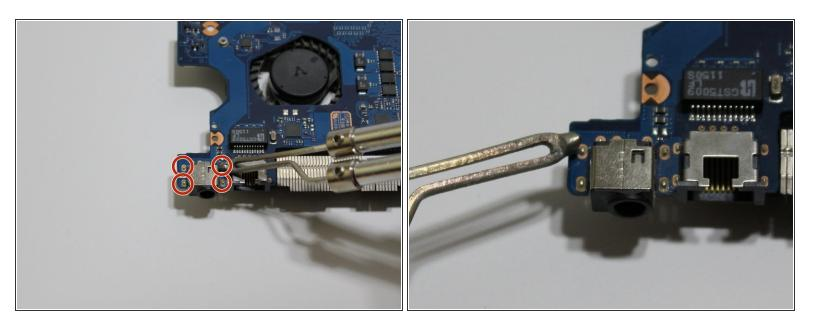
• Using the Soldering Station, remove the power jack from the four connectors.
