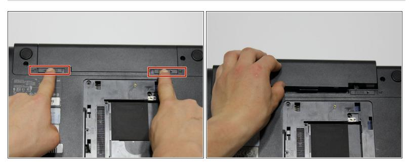
Remove the battery by pushing out the locks on either end then pushing the battery away from you.
