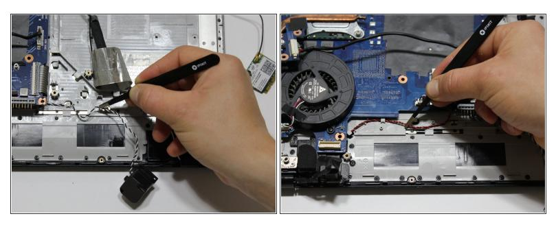
Using the blunt tweezers, unthread the wires that connect the motherboard to the speakers from their holders, without crimping the wires.
