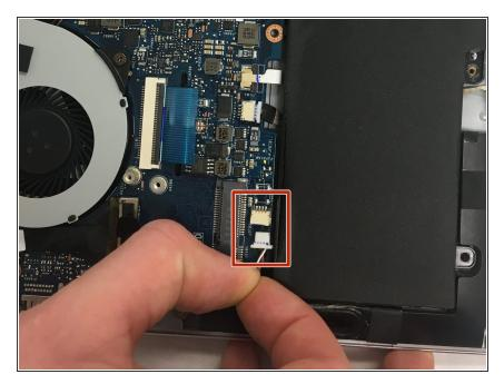
Disconnect the speaker by carefully pulling the speaker cable away from its socket on the motherboard.
