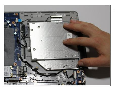
Remove the disc drive by pulling it towards the outside of the computer.
