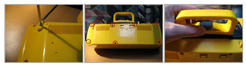
Start with Removing the Antenna by unscrewing the single screw. Then Unscrew the Seven Screws on the Back of the Radio as indicated in the Photo. Then remove the handle by simply unscrewing the knob in the middle.
