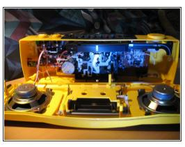
Remove the two screws located under the Stereo Handle. Now, Wedge open the front of the box.
