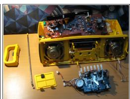
• Undo the retaining clip from the Board. Make sure when Wedging upward the Radio receiver wheel is in good shape on the right of the board- and remember to realign during reassembly. Lean board upward. This is as far as i am going to go with this project because the wires below the board are soldered. Fun Fun Bladow! - Sony Stereo-Corder in a organized pile of heap.
