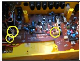
Now to remove the tape mechanism. The buttons are gloved so your gonna have to wedge them out of their sleeves. Then when removed from rubbers. Unattach the three (circled in yellow) flat cables connected to the board.
