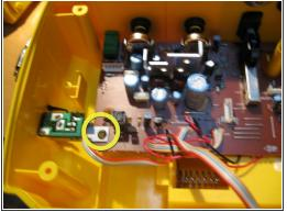
• Disconnect the Flat Cable that stems to the Speakers. Remove The Screw on the right, then the Middle, then the one on the left of the MainBoard. The left one has a little supporting metal piece, remove that as well.
