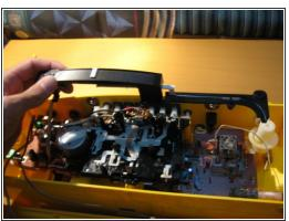
Unscrew the Single screw under the tape mechanism. Gently pop out the Radio tuner indicator lever and put to side- Do not attempt to remove this piece, it is soldered to the front face leds
