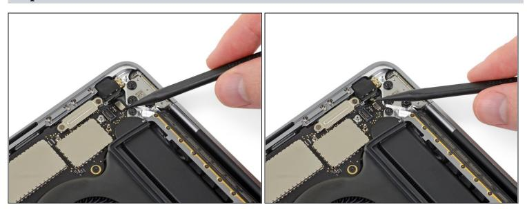
• Disconnect the power button and Touch ID sensor by prying its connector straight up from the logic board.
