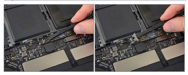
Use a spudger to gently lift the battery power connector, disconnecting the battery.
