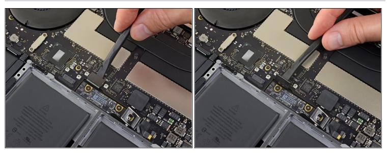
• Use your spudger to disconnect the keyboard by prying its connector straight up from the logic board.
