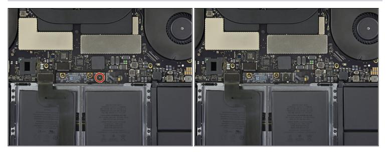
• Use a T5 Torx driver to remove the 3.7 mm pancake screw securing the battery power connector.
