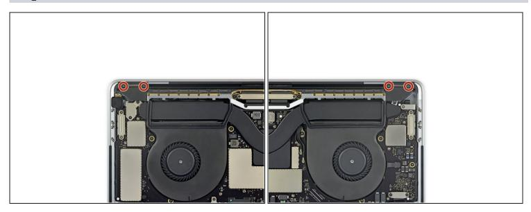
• Use a T3 Torx driver to remove the two 2.0 mm screws securing each hinge cover (four screws total).
