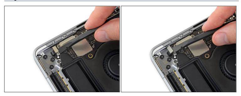
• Disconnect the Touch Bar digitizer cable by prying it straight up from the logic board.
