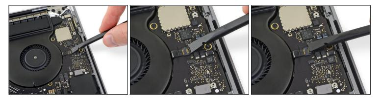
• Open the locking flap on the microphone cable's ZIF connector by prying it straight up from the logic board.
