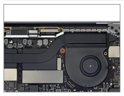
Use a T5 Torx driver to remove the single 2.9 mm screw securing the antenna cable bundle.
