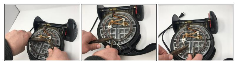
• Use two pairs of needle-nosed pliers to pull the fuse out of the conduction bearing. Firmly grasp one end of the thermal fuse with one set of pliers and the conduction bearing it is connected to and pull them apart.
