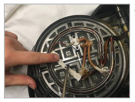
Secure the thermal fuse by reattaching the clasp and screwing it into place.
