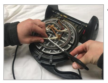
Cut through the insulation to expose one end of the thermal fuse using a pair of scissors.
