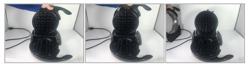
• Pull the handle up and away from the waffle iron to remove the cover and expose the circuit.
