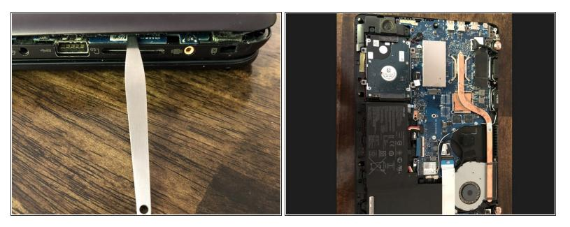
(i) Use the prying tool to help maneuver and separate the back plate off of the computer safely. This will expose important hardware and internal parts.
