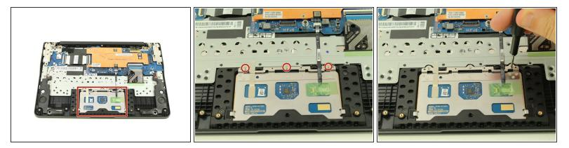
• Remove the three 2.3mm screws along the top of the trackpad using a Phillips #00 screwdriver.
