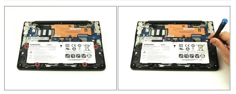
Locate the battery and remove the four 4.6mm screws at the corners which attach it to case using a Phillips #00 screwdriver.
