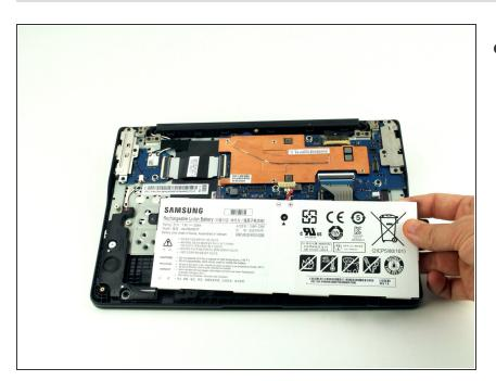
• Lift the battery up and out from the case.
