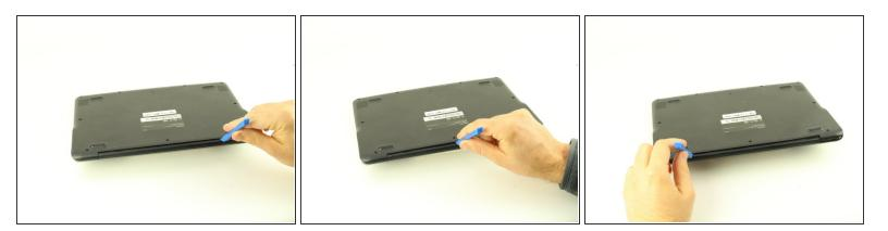
• Use a iFixit opening tool to gently pry the case up from the vent on the hinge side of the Chromebook.
