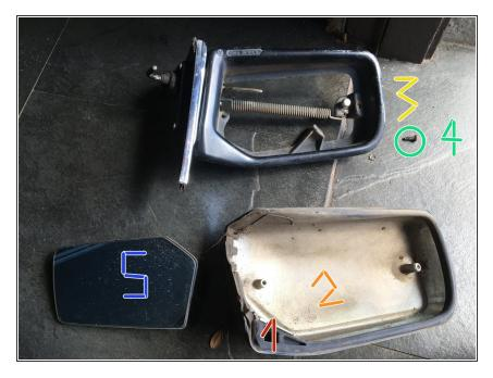
To reassemble follow the instructions in reverse order: place the rubber gasket (1) in the chrome cover (2), assemble with the black aluminum body (3), fasten the Phillips screws (4), slide in the mirror (5) to the arm and push firmly to secure the metallic pin in the plastic socket.
