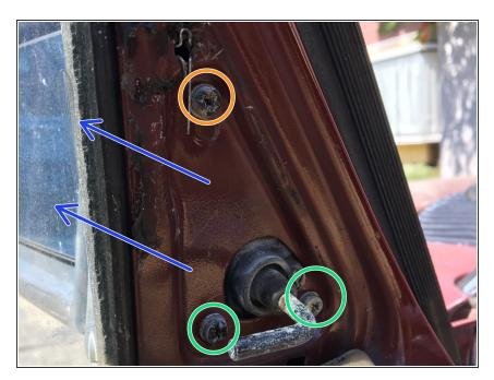
• Remove the 3 Philips screws that hold the mirror in its place. It's best if you remove the ones located in the bottom first, then, holding the mirror, remove the last one. The idea is to avoid the mirror from falling to the ground.
