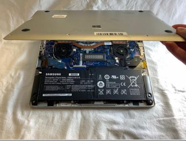
Gently lift and remove the bottom case.
