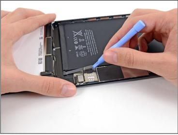
• Use a plastic opening tool to gently pry the battery connector up from its socket on the logic board.
