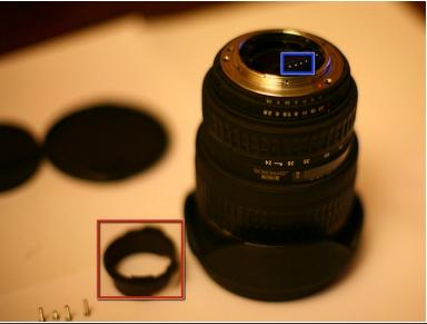
Remove the 4 screws around the steel ring in order to disassemble the captor (blue area) and the plastic ring (red area) which is insert inside the steel ring and behind the captor
