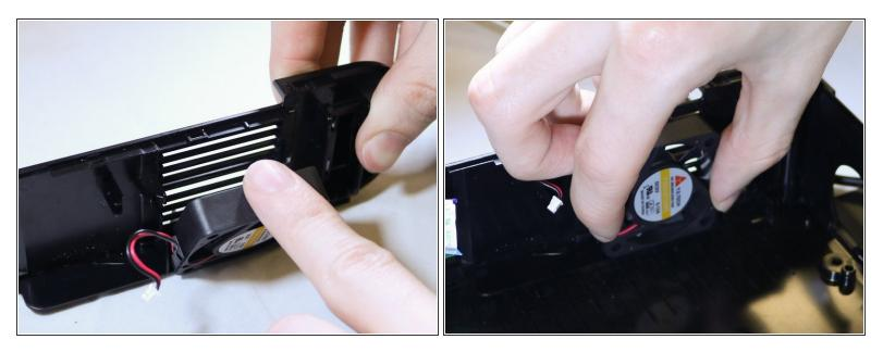
• Remove the fan by tilting it forward slightly and then lifting upwards.
