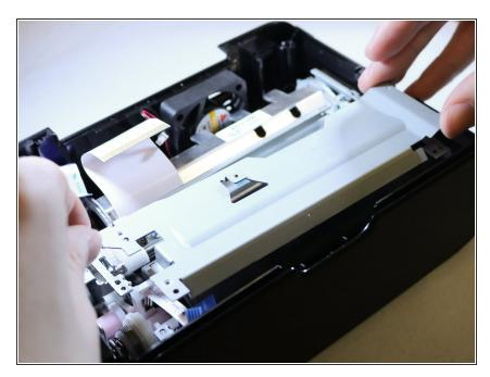
• Lift out the print mechanism of the printer case.
