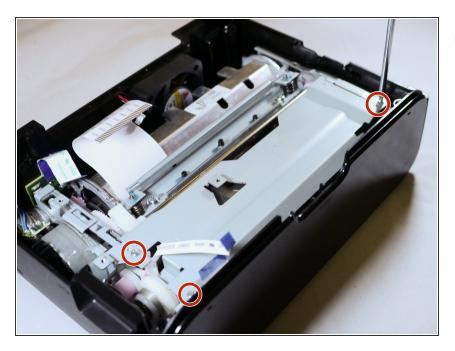
Unscrew the three 3mm PH000 screws securing the metal plate to the printing mechanism.
