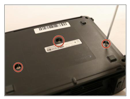
• Unscrew the three 4mm PH1 screws on the bottom of the printer.
