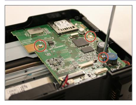
• Unscrew the three 3mm PH000 screws from the motherboard.
