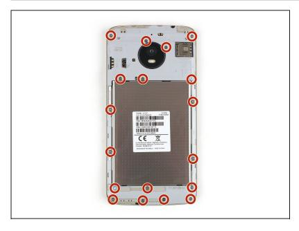
Remove the eighteen 3.3 mm Phillips screws securing the midframe assembly.
