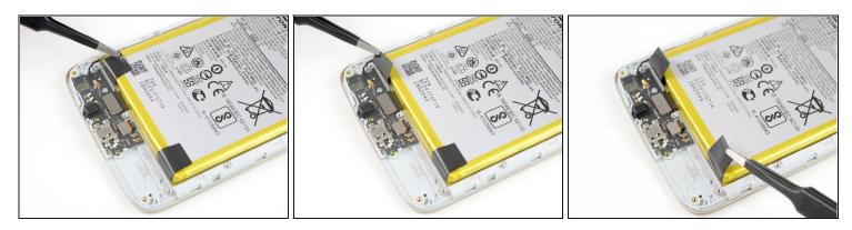
• Use a pair of <u>tweezers</u> to peel the ends of the two pull tabs off of the bottom edge of the battery.
