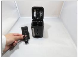
Press the mounting plate button and slide upwards.
