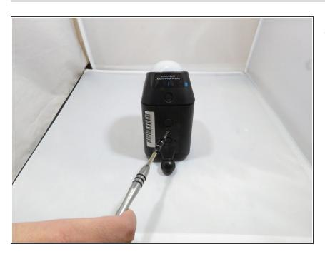
Remove the screw using the screwdriver and head tool PH00.
