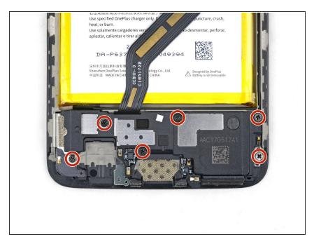
Remove the six 2.6 mm Phillips screws securing the loudspeaker to the frame.
