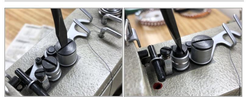
Adjust the thread pull-off lever as well as adjust the position of the nipper bar block to the left or the right.
