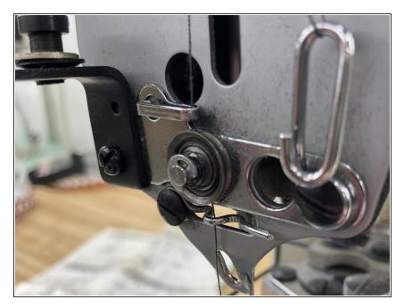
Again, keep the thread along the groove of the wheel before slipping it through the eye of the needle.
