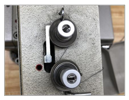
Loop the threading through the two tension posts, making sure you stay in the grooves of the wheels.
