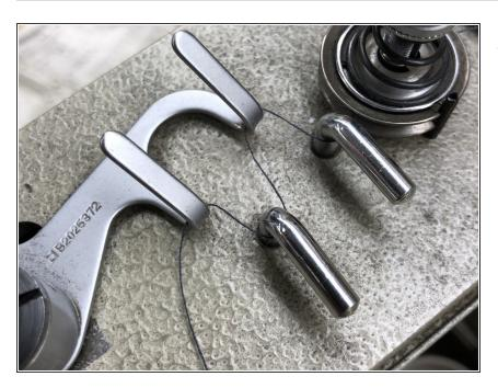
Continue the threading, weaving through the pull-off lever.
