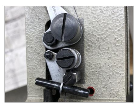
Tighten the thread on the top loop near the nipper releasing knurled thumb nut.
