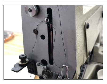
Weave threading through the working arm and have it ready to insert through the eye of the needle.
