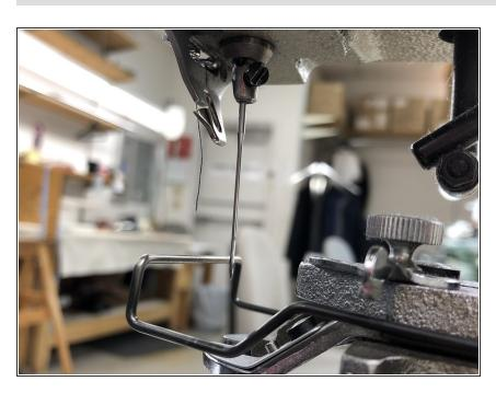
Using the flathead screwdriver, slide the needle up into the slot, with the indented side facing in and tighten until the needle cannot shift.
