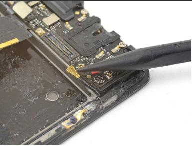
Slide the point of a spudger underneath the antenna interconnect cable and pry up, disconnecting
