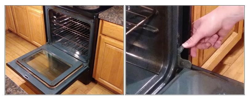
• Open the oven and unlock hinges that are located at the bottom of each side of the oven.
