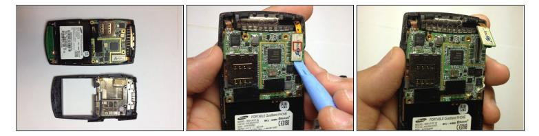
• Use the prying tool to disconnect the rectangular connector.
