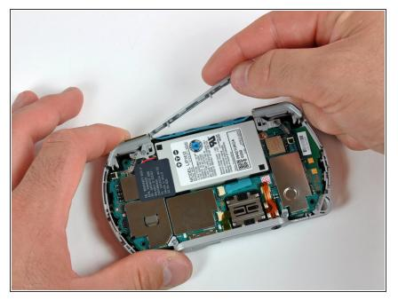
• Pull the top cover upwards gently from its housing.
