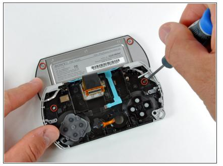
• Use a #00 Phillips screwdriver to remove the four display screws.
