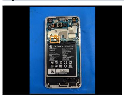
Disconnect the battery. While holding the motherboard down, pry up on the battery connector.
