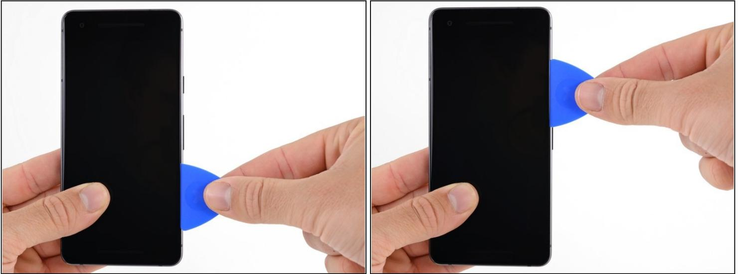
ⓘ In the following steps, use the flat of the opening pick, rather than a corner, to cut here. This will help prevent inserting the pick too deeply.
